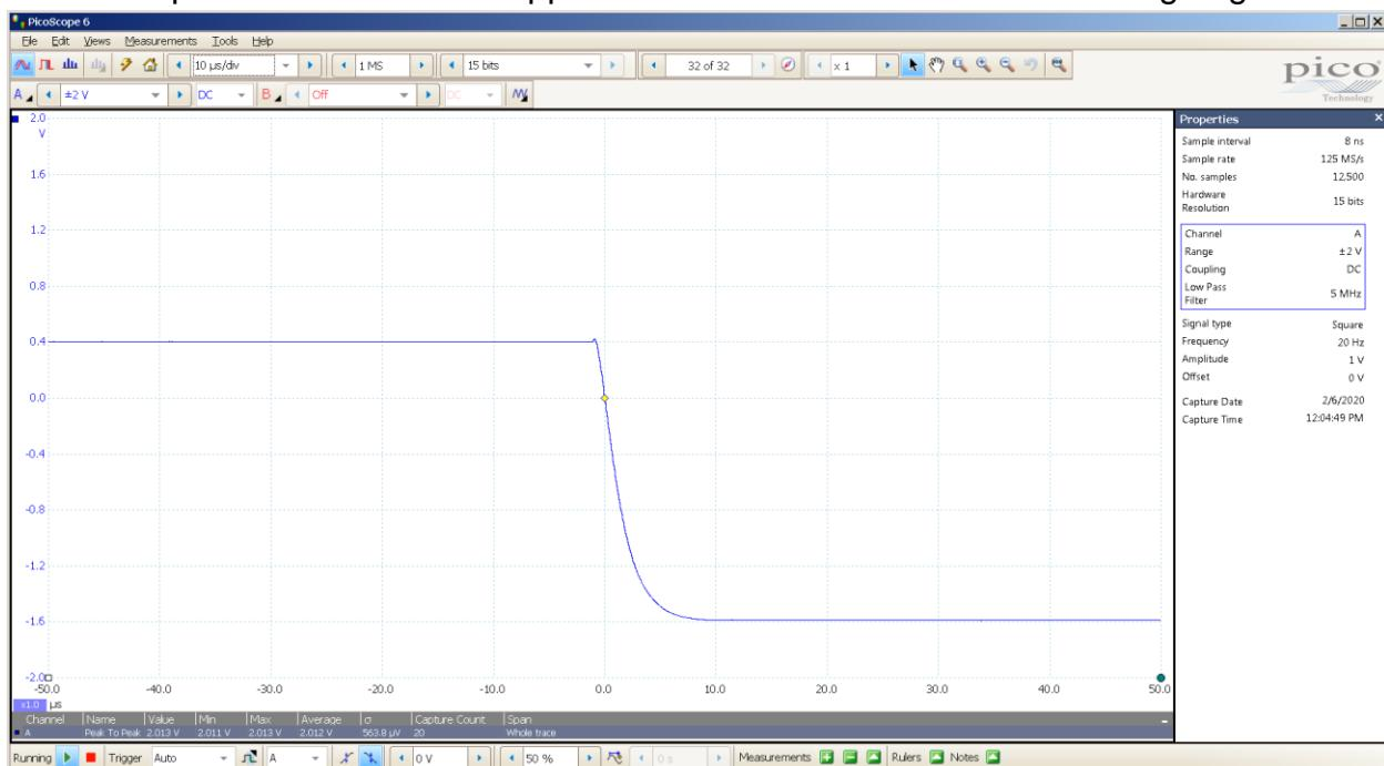
ECP Audio T4 SE input SE Output square wave measurements
