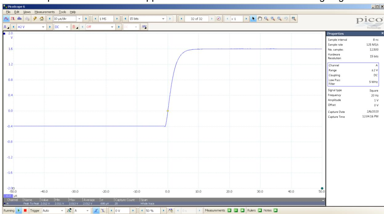
ECP T4 square wave 20 Hz 2 Vpp 10 uS / div 32R load 5 MHz BW falling edge
