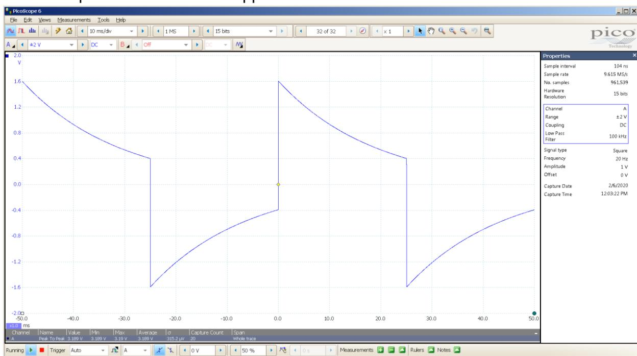
ECP T4 square wave 20 Hz 2 Vpp 10 mS / div 32R load 5 MHz BW
